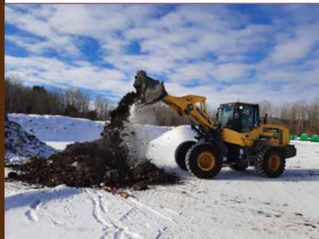
Our "new" organics loader is also used, but prevents delays in compost windrow management due to competing with recycling and waste transfer for loader time.
